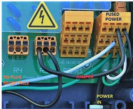
Figure 25 Wiring R3 using on-board fused power
