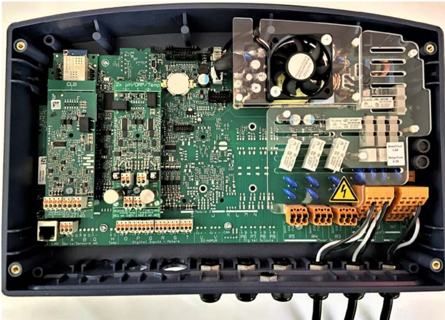
Figure 35a Overall view of the DCM3 interior with both driver cards as factory installed
