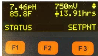
Figure 4 Typical Home screen no alarms
