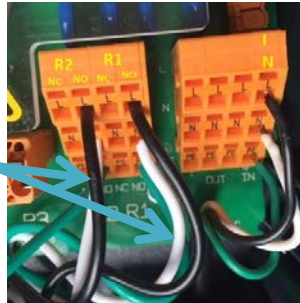
Figure 23 Terminating R1 & R2
