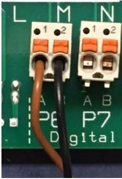
Figure 29E Concept pump cable on Output Relay P6 (Enable/Disable-ON/OFF Mode)
