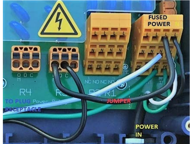
Figure 25 Wiring R3 using on-board fused power
