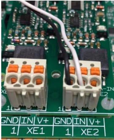
Figure 57 Two wire remotely powered analog input
