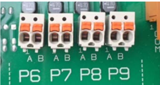
Figure 29A Digital DC outputs 6-9
