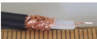
Figure 50B Coax cable preparation with conductive sleeve removed
