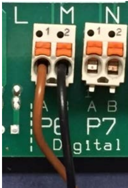
Figure 29D Universal Control Cable on Output Relay P6 (Enable/Disable-ON/OFF Mode)
