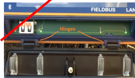
Figure 65 USB Access Door Closed [Top] and Open [Bottom]
