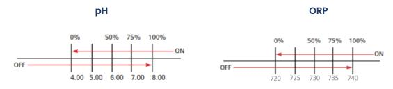
3) Fixed PWM Mode- controls how much the chemical pumps to get to the setpoint and how fast it is pumped into the pool. This mode lets you tell the controller how long to pump chemicals into the pool and how long to stop pumping chemicals into the pool before it starts pumping again. \*It is very normal for the chemical pump to stop pumping while in fixed setting. It will run for a length of time and stop for a length of time you set. Ton:40 seconds WORK Toff: 10 seconds PAUSE
