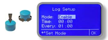
Log activity recording can be started by moving wheel on "Mode: Disable" and changing it to "Mode: Enable". Log activity starting time can be set to begin at specified time by entering "Time". Activities data are collected every specified hour or minutes. Edit this parameter by moving wheel on "Every: 00:00" and changing it to desired time.
