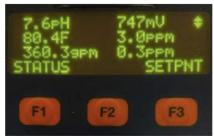
Setpoint is the ideal point where the chemical controller stops pumping chemicals. Example: if you set PPM to 3.0 the chemical controller will pump until 3.0 and turn off.
