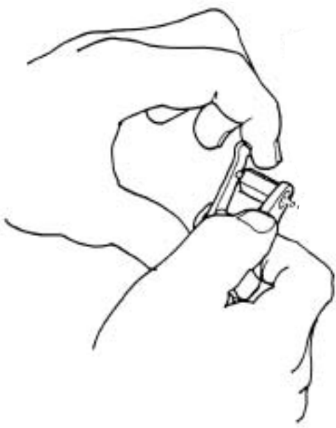
LIFTER, HOLDER, AND INDEX PIN WITH CARBIDE TIP (SPRING IS ENCLOSED)
