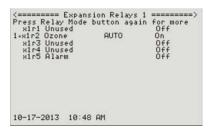
By selecting one of the assigned relays, you are allowed to choose between automatic, manual on or manual off. Unused relays and the alarm relay cannot be manually overridden, but their current state is always displayed.
